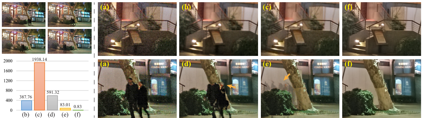
Figure 1: Top-left: a burst of noisy images (10 frames with image size 3072 \times 1728 ) by a smartphone. Bottom-left: the running time (sec.) of different denoising methods. Right: comparison of two close-up views. (a) input images (b) spatial-temporal filtering [Bennett and McMillan 2005] (c) BM4D [Maggioni et al. 2013] (d) optical flow [Liu 2009] + median (e) lucky imaging [Joshi and Cohen 2010] (f) our method. Our method produces a clean, ghost-free image with fine details. More importantly, our method is significantly faster than other methods.
